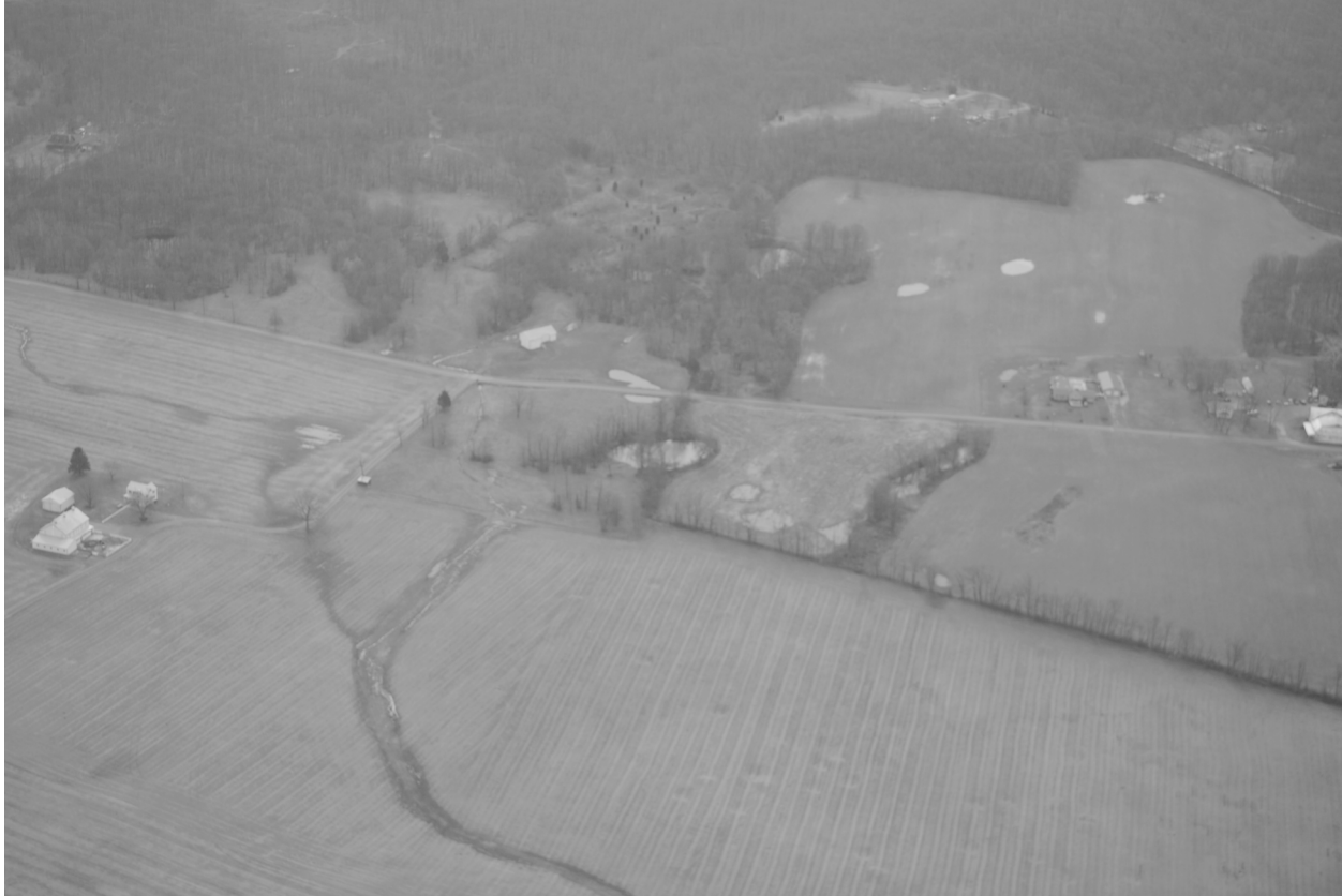
Figure 47. Aerial view of Walnutdale Road at Mile 52.1 in mid-March, 2011 after heavy rain. Note numerous karst depressions full of water.
