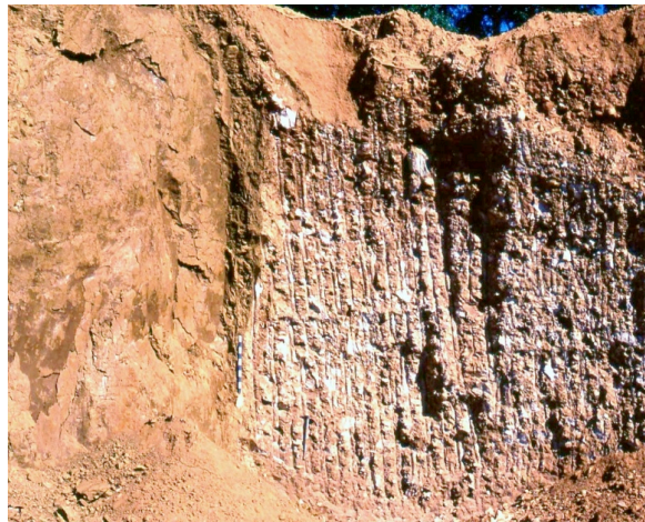
Figure 55. Contact of sand plug (left) and colluvium (right). Scale divided into 10 cm intervals. Note slickensided clay at contact.
