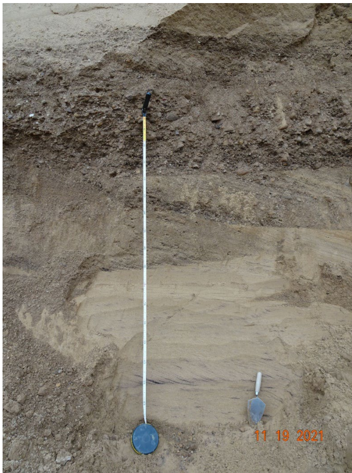
Figure 5.7. Close up of location of OSL sample 11-19-21-1 in asymmetrical ripple cross laminated sand. Coal is dark material that accentuates ripple laminations. Scale is 1.7 meters.
