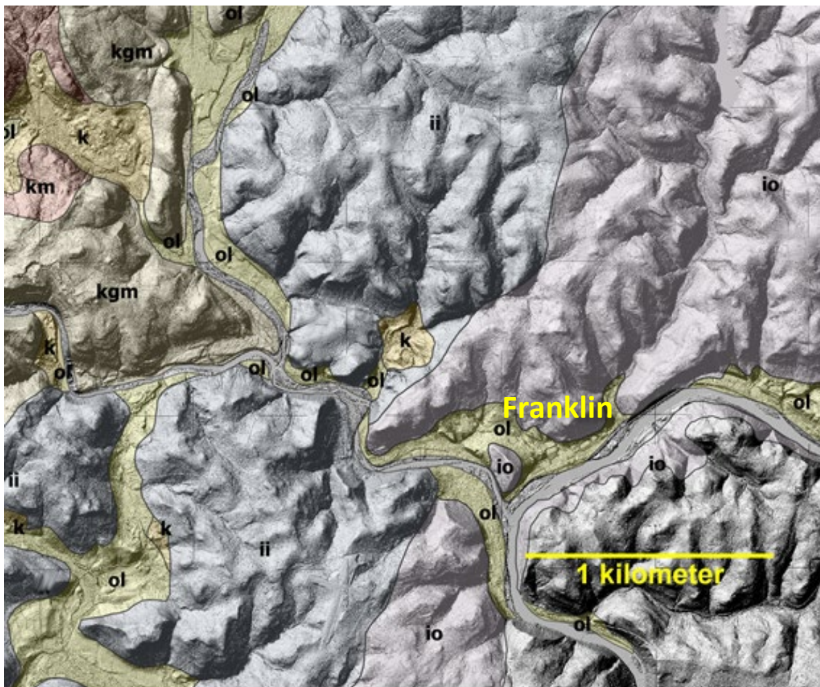
Figure 5.1. The Vincent and Cooperstown pits are located in the kame deposit (k) in the center of the map. The ii is the mapped extent of Titusville Till. io is Mapledale Till. km and kgm are Kent Moraine and ground moraine, respectively. Outwash is labeled ol. Geology from Shepps et al (1959), Plate 1 overlain on 10x lidar hillshade.
