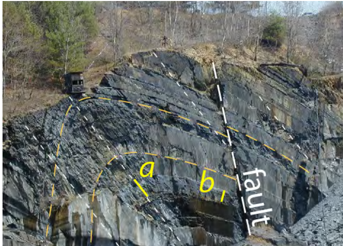
Figure 6. Close-up of anticline hinge area showing the difference in the length of a piece of slate that could be derived from the same bed in the hinge area (a) and on the limbs (b). In this case the length in the hinge is 180 percent greater than in the limb.
