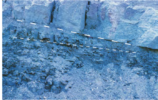
Figure 3. Contact between the Shawangunk (above) and Martinsburg Formations along I-84. The angular difference between bedding in the Shawangunk (long dashes) and Martinsburg (short dashes) is 5°. Picture taken June 1966.
