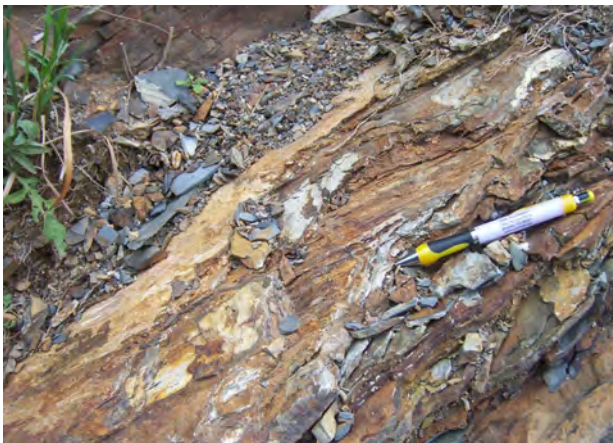
Figure 9: Bedding plane slickensides in the Martinsburg about 10 ft (3 m) below the contact with the Shawangunk formation. Pen points in direction of movement to the lower left.
