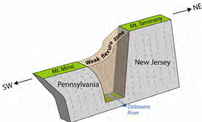
Figure 16. Reconstructed flexure at Delaware Water Gap. Dotted line shows strike of beds before the gap was cut. The flexure accounts for the offset of the ridge between the two sides and presumably resulted in considerable fracturing of the Shawangunk at the gap site. View looking eastward. The flexure also explains the offset of the Kittatinny Mountain ridge between the two sides of the gap. Graphic by Trista L. Thornberry-Ehrlich (Colorado State University) after Epstein (2006, fig. 9).
