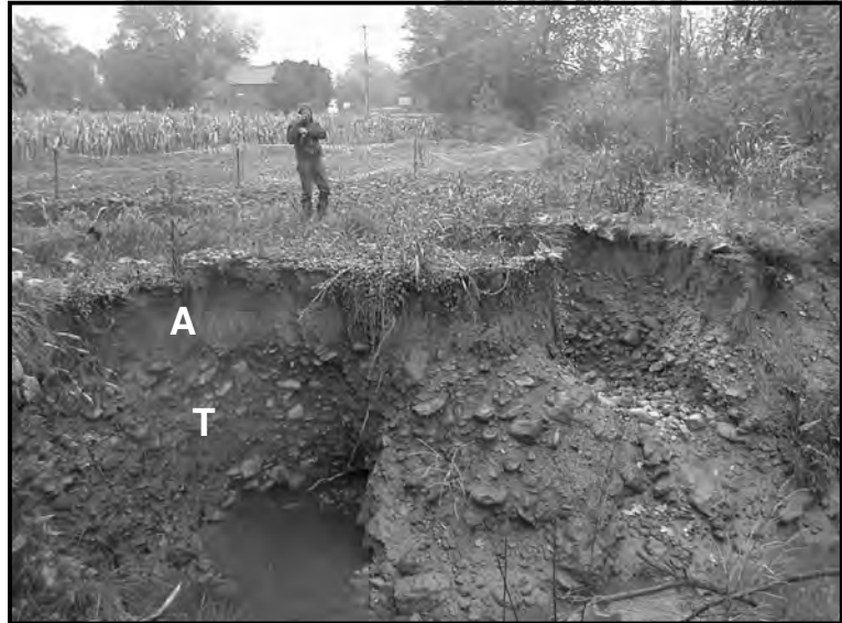
Figure 3. Sinkhole along the north bank of the Bushkill Creek showing coarse glacial till (T) overlain by finer alluvial sediment (A)
