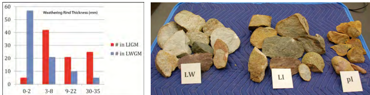
Figure 20. Left— Weathering rind thickness on clasts collected from stone rows near Riverton, PA (LWGM deposits) and near Mud Run (LIGM deposits). Clasts labeled 30-35 mm are actually weathered throughout the interior; Right— Examples of samples represented in Figure 20a. Note the relatively fresh nature of specimens labeled as late Illinoian relative to those labeled pre-Illinoian. The labels are situated on a Bloomsburg clast for comparison for each group.
