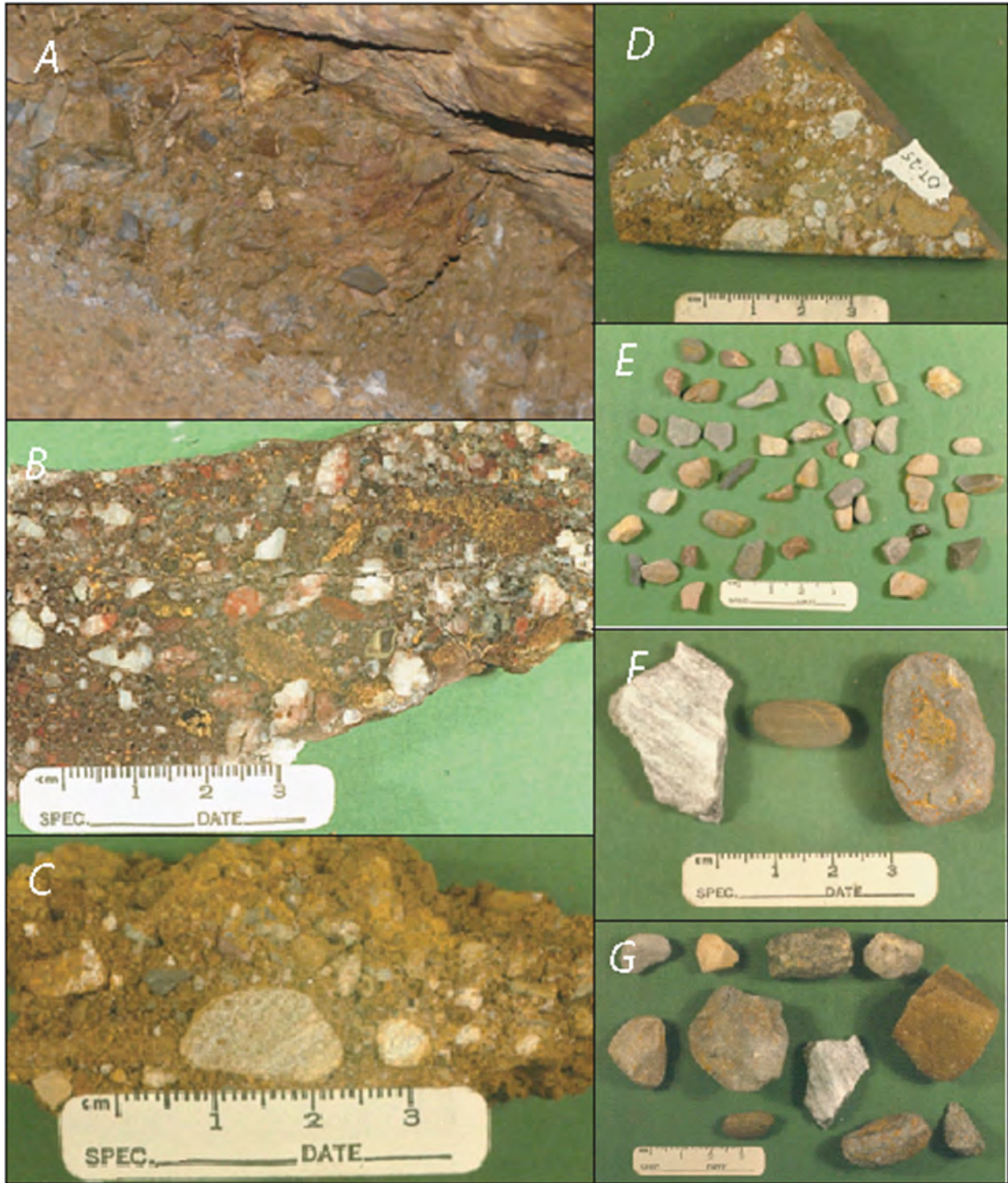
Figure 4. A—Diamictite between the overhanging conglomerate of the Shawangunk Formation and shales of the Martinsburg Formation; B, C, and D—Chunks excavated for the diamictite showing light-colored sandstones, red beds, and dark shales; E—Variety of shapes of the pebbles; F—Some pebbles are rounded, others are angular, such as the slickensided white quartz vein material on the left; G—Sandstones, siltstone, and slickensided vein quartz in a variety of shapes.
