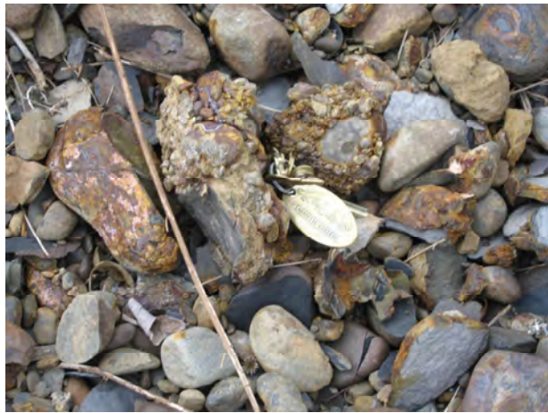
Figure 15. Fresh to lightly weathered shales and siltstones in kame pit north of Saylorsburg, PA.
