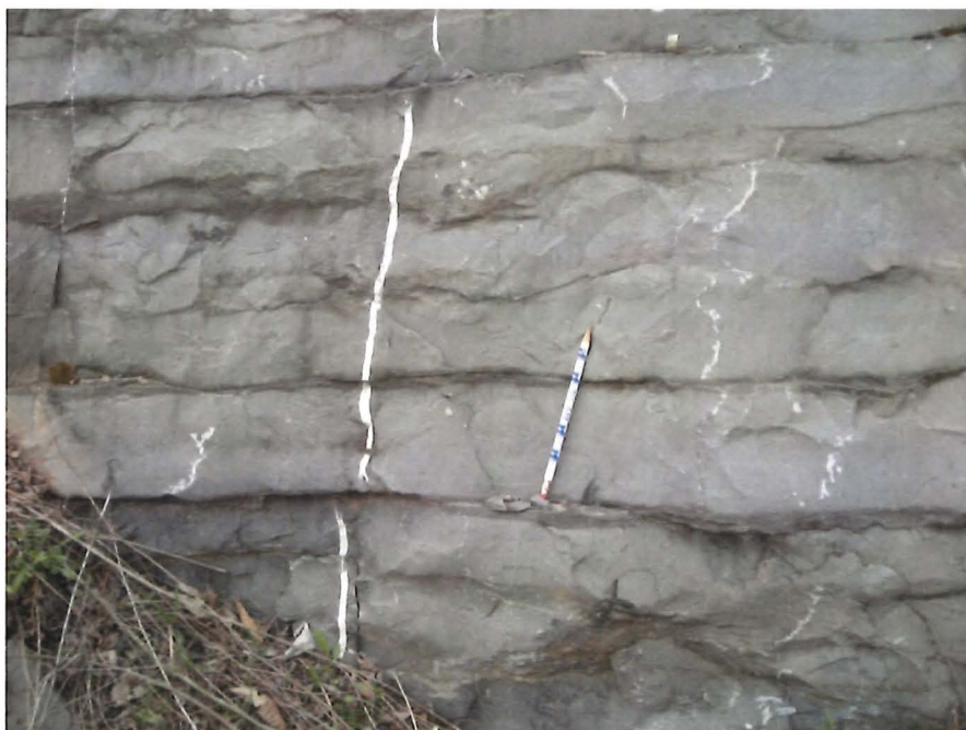
Figure 2. Dickinson College Quarry, showing shaly partings along which rocks break, and a thin calcite vein. Pencil for scale.
