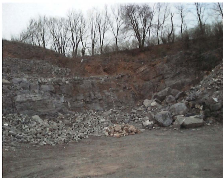
Figure 1. Dickinson College Quarry, looking South. Note gentle dip down to left and thin partings along which rocks weather and break.
