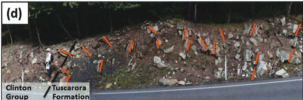
Fig 6. (d) Location 3 on Figure 4, looking northeast (approximately along bedding strike). Tuscarora sandstone at right is mostly in place, dipping northward (to left), but downslope to left slabs of sandstone become increasingly rotated to the north, with greater amounts of rotation near the ground surface at top. To left of the contact with the Clinton Group is colluvium with no discernible in-place bedrock, part of a solifluction lobe that can be traced across the road and downslope. Gray-black material to right of person (1.56 m high) is asphalt rubble.
