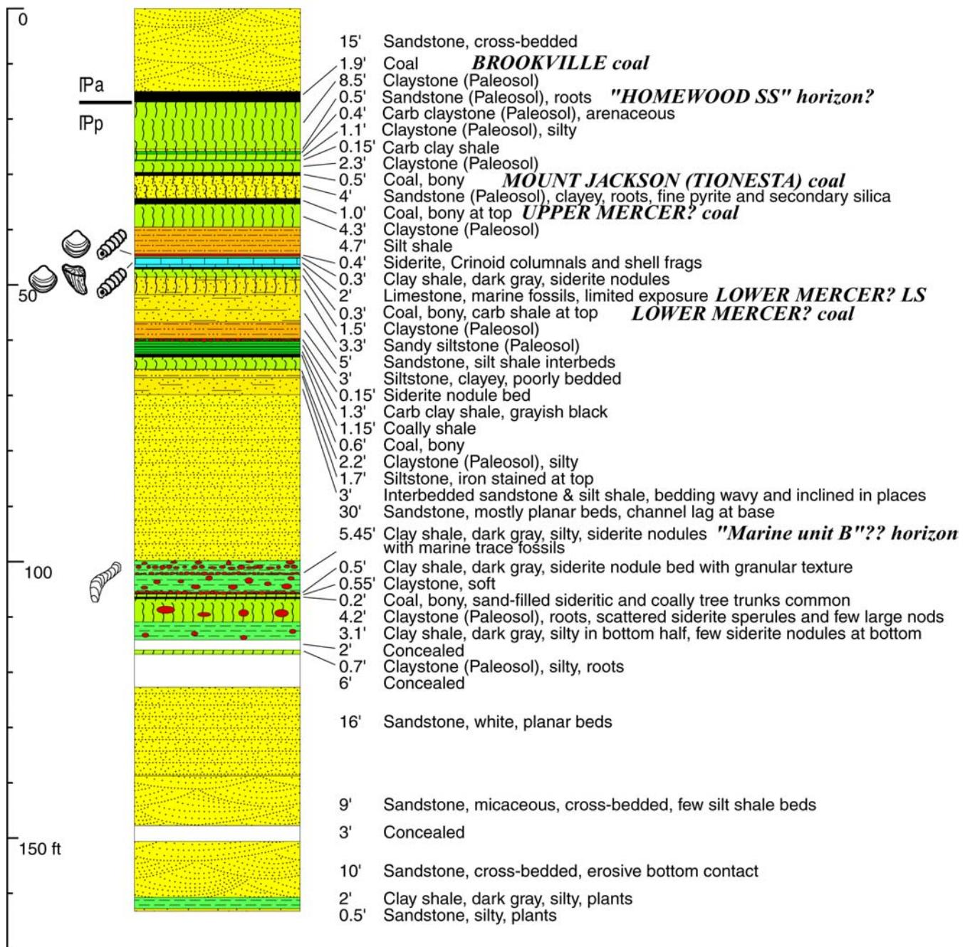
Figure 12-2. Geologic section of rocks exposed at US 422 and Toll 60 interchange. "Marine unit B" and lower rocks were measured in stream cut a short distance southeast of the Toll 60 North exit ramp road cuts.
